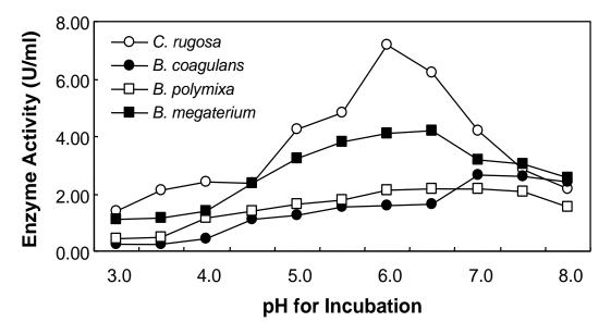
Figure 2. Effect of pH on enzymatic activity of microbial.CGTase.
