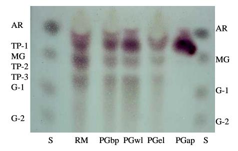
Figure 4. Thin layer chromatogram of transglycosylation reaction products. Transfer products (TP-1, TP-2, TP-3) before purified (PGbp) and after purified (PGap) were detected in the presence of aglycone in accordance to standard solution (S) containing Maltose (G-2); Glucose (G-1); Methyl □-glucoside (MG); Arbutin (AR).
